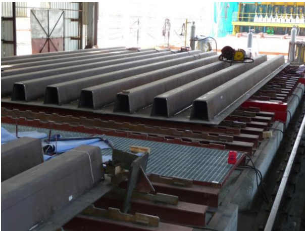
Figure 10. Deck Panel Fabrication
